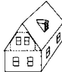
(F) 1 1/2 Story. This type has a high pitch roof with a slope of about \frac{5}{8} or \frac{3}{4} with small dormers on one or both sides of the roof. The area of the finished second floor is approximately 75% of the first floor area.
